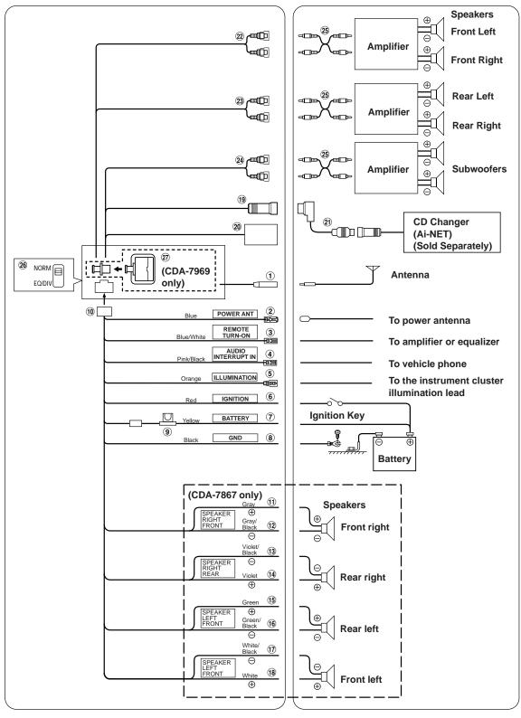
For details on how to set the Subwoofer to ON/OFF, see "Subwoofer On and Off" on page 6.
